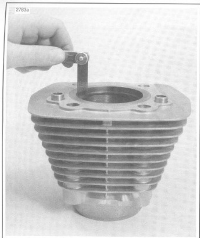
Figure 3-31. Measuring Ring End Gap
