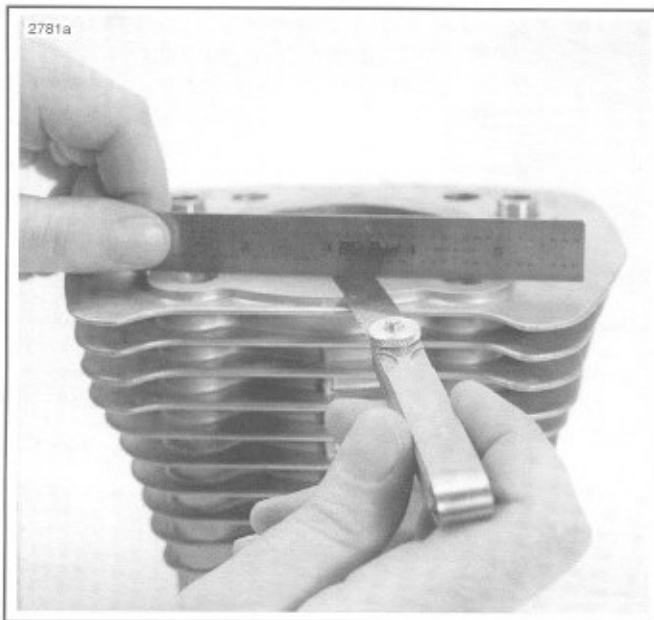
Figure 3-28. Checking Gasket Surfaces
