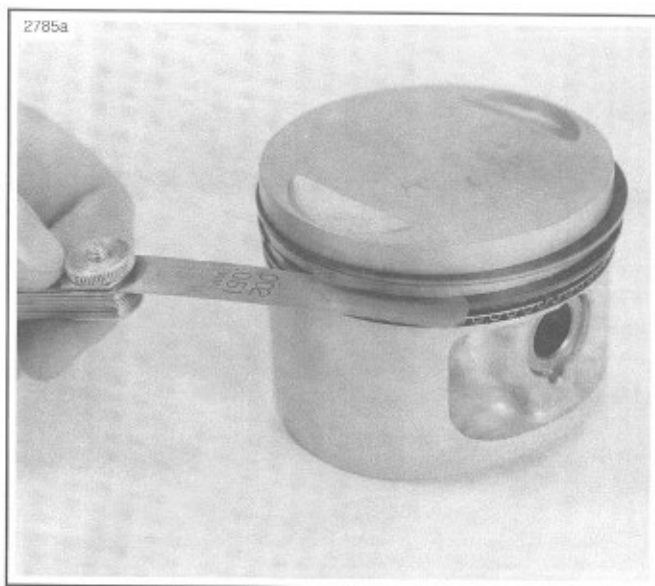
Figure 3-34. Measuring Ring Clearance in Groove
