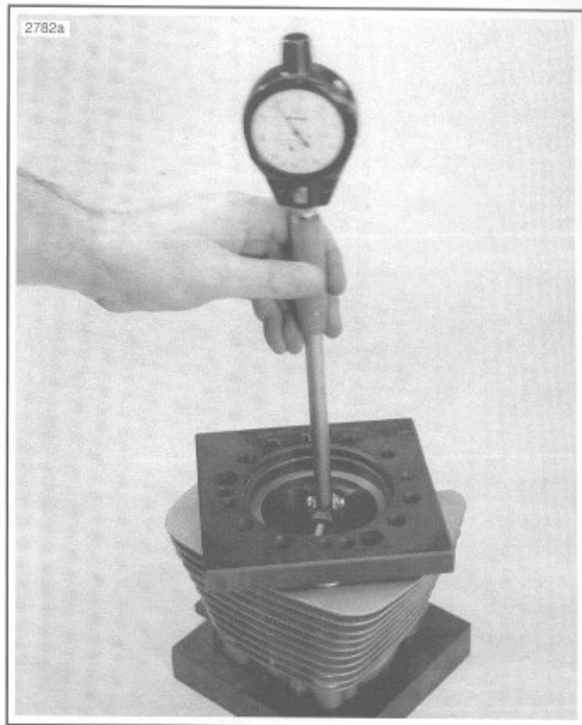
Figure 3-29. Measuring Cylinder Bore
