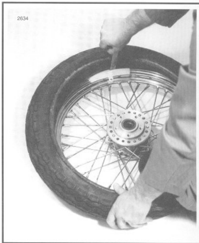
Figure 2-35. Starting Bead on Rim
