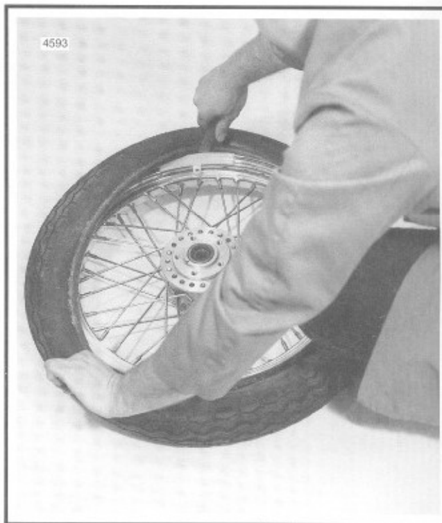
Figure 2-36. Starting Second Bead on Rim
