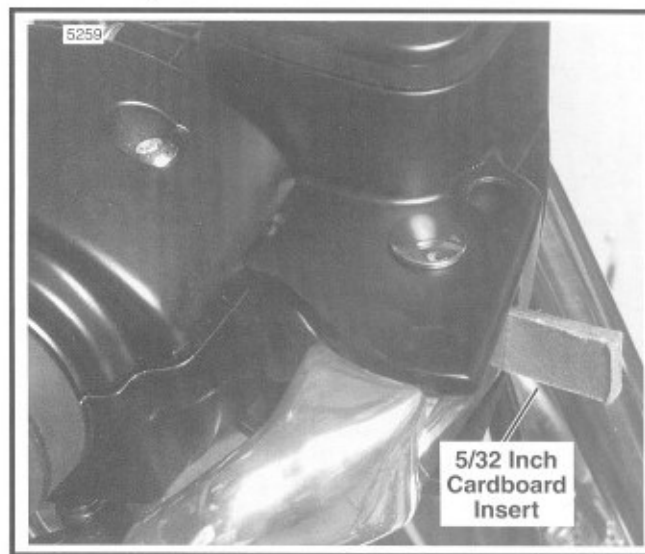
Figure 2-43. Install Cardboard Insert Before Removing Master Cylinder Assembly
